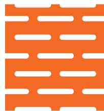
S1931SR 19 x 3.2mm Slots @ 11.12 x 6.4 mm Centres 41% Open Area
