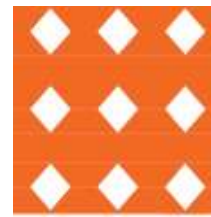
S5512SD 5.56mmSq Diag x 12.7mm Pitch 19% Open Area
